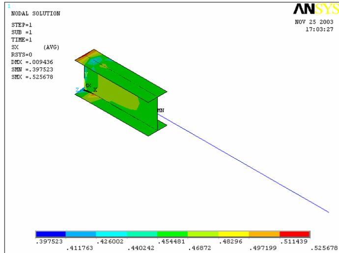
Fig. 6-4 Normal Stress Distribution of Cantilever without RBS under Axial Load
