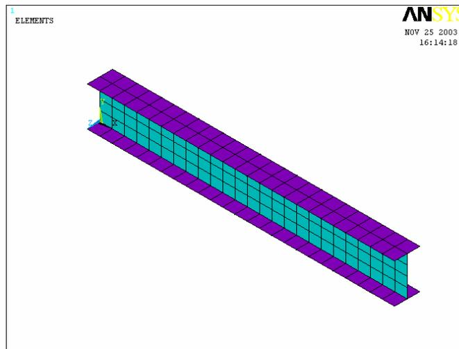
Fig. 6-2 Full Shell Model of Cantilever Beam without RBS
