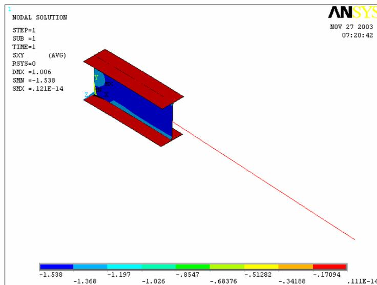
Fig.6-7 Shear Stress Distribution of Cantilever without RBS under Transverse Load
