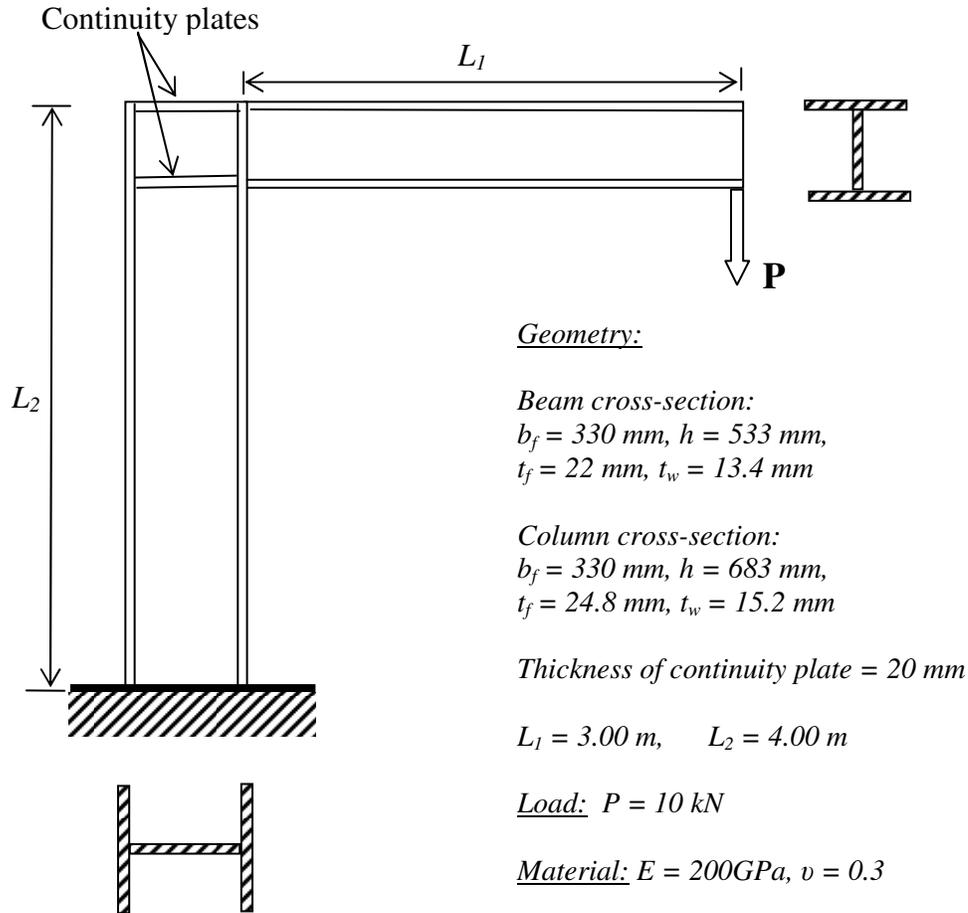
Fig. 6-19 Example 2: Inverted L-Frame
