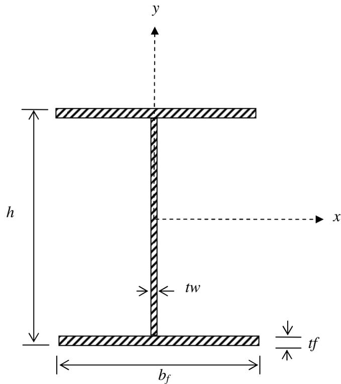
Fig. 5-1 Cross-sectional Parameters of I Beam Section
