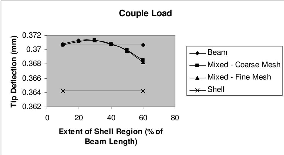
Fig. 6-10 Tip Deflection vs. Extent of Shell Region for Couple Load
