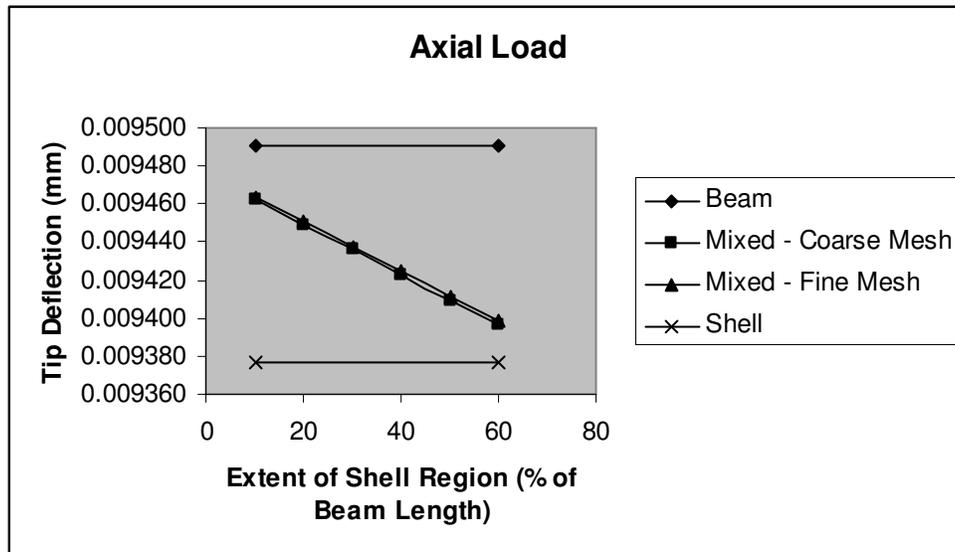
Fig. 6-9 Tip Deflection vs. Extent of Shell Region for Axial Load
