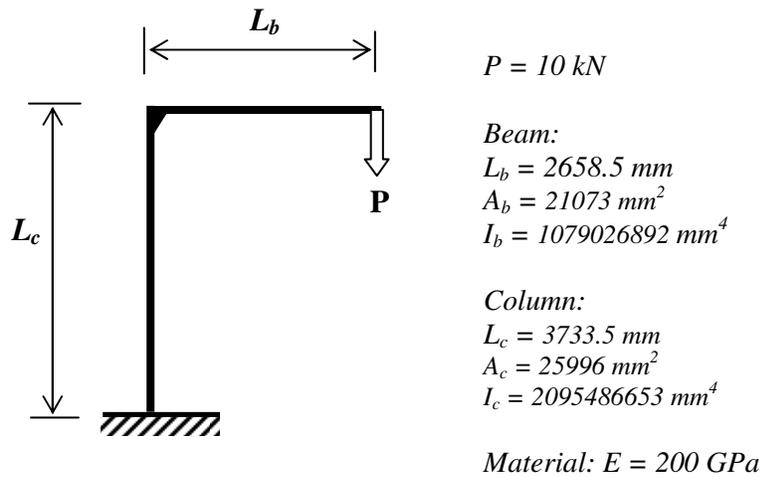
Fig. 6-25 Frame Model of Inverted-L Frame
