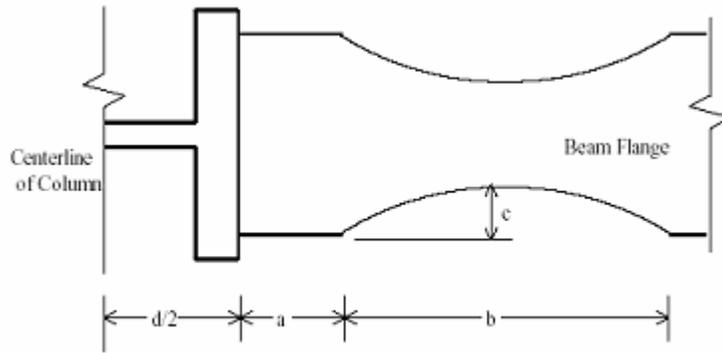
Fig. 2-5 RBS Geometric Parameters
