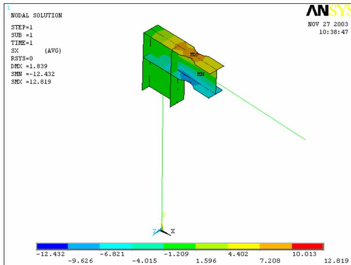
Fig. 6-28 Normal Stress Distribution of Inverted-L Frame with RBS
