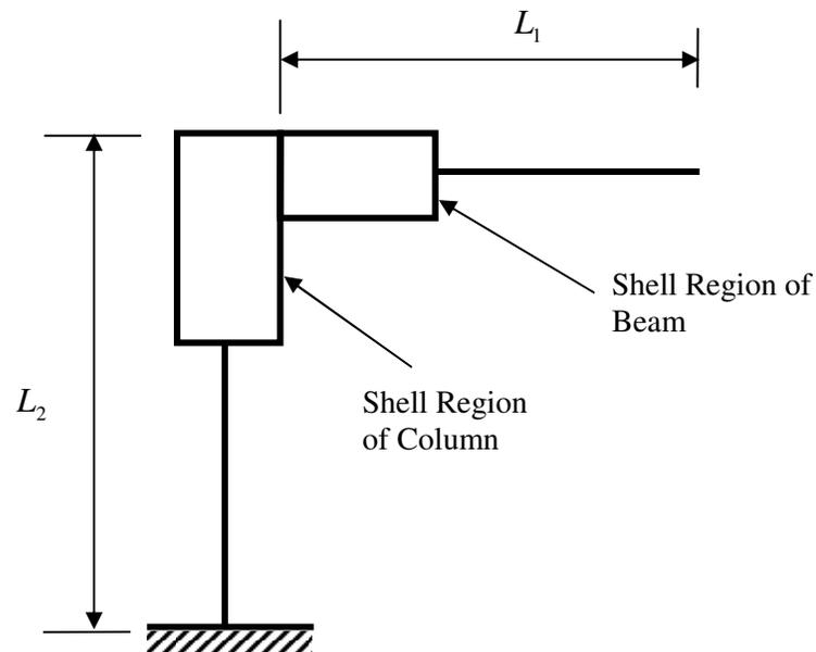
Fig. 6-21 Extent of Shell Regions in Beam and Column
