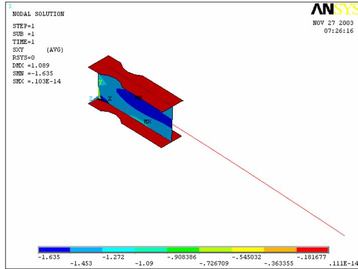
Fig. 6-18 Shear Stress Distribution of Cantilever with RBS under Vertical Load
