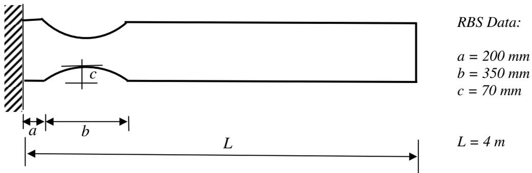
Fig. 6-12 Cantilever Beam with RBS
