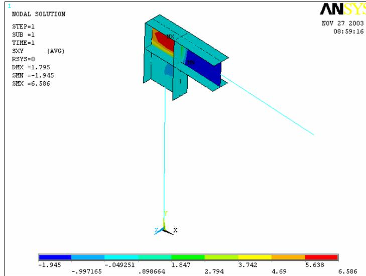
Fig. 6-24 Shear Stress Distribution of Inverted-L Frame
