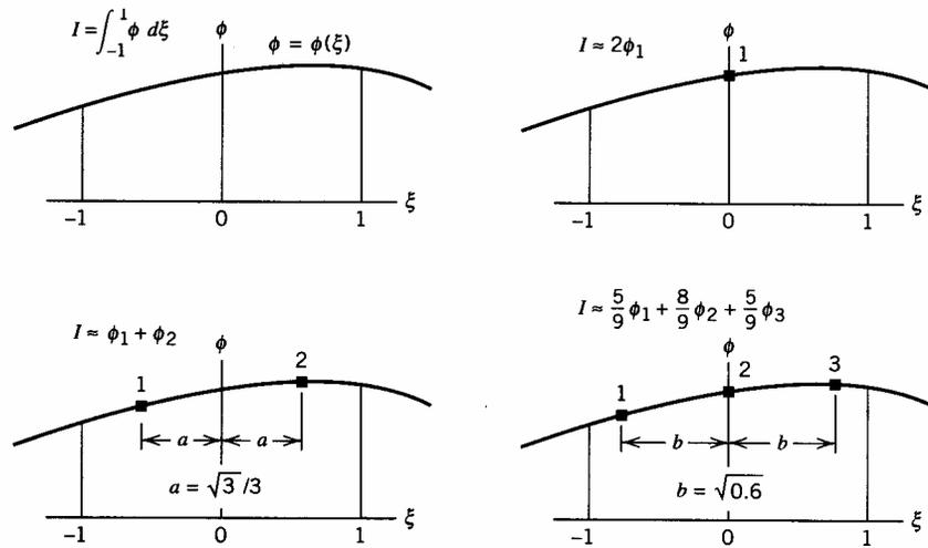
Fig. 3-2 One Dimensional Gauss Quadrature of Orders 1, 2, and 3 [10].
