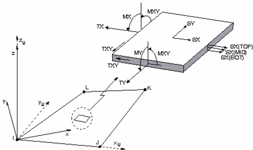
Fig. B-2 SHELL63 Stress Output
