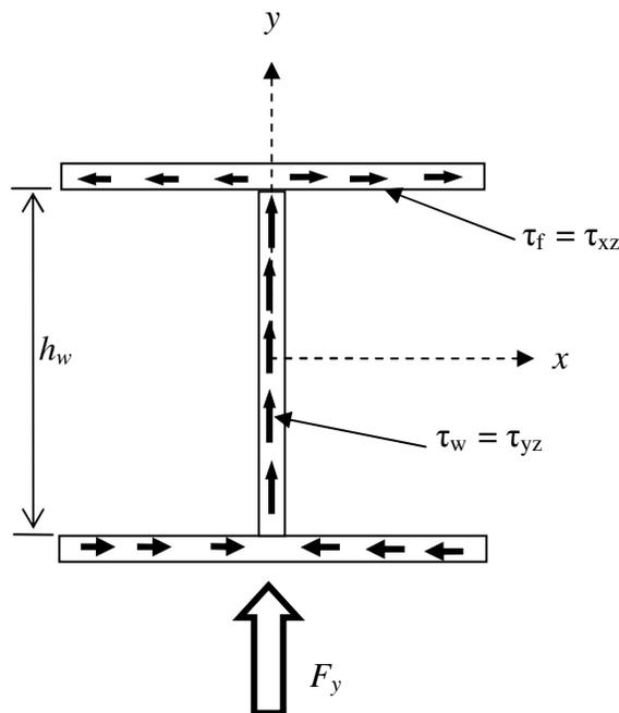
Fig. 5-5 Shear Stress Distribution due to Force in the Y-direction
