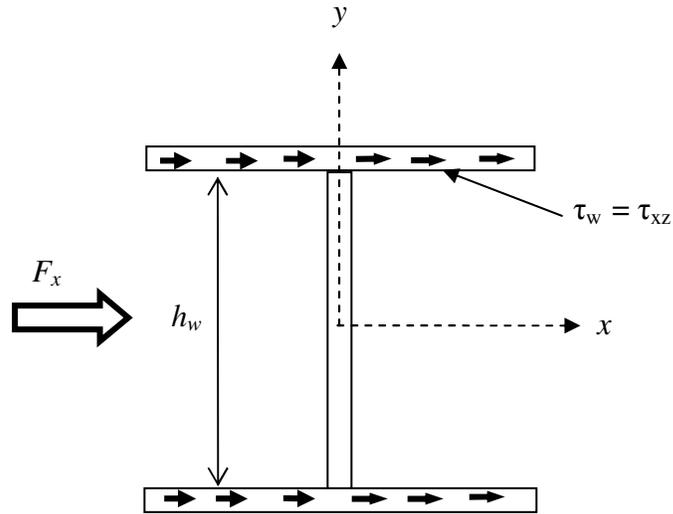
Fig. 5-6 Shear Stress Distribution due to Force in the X-direction
