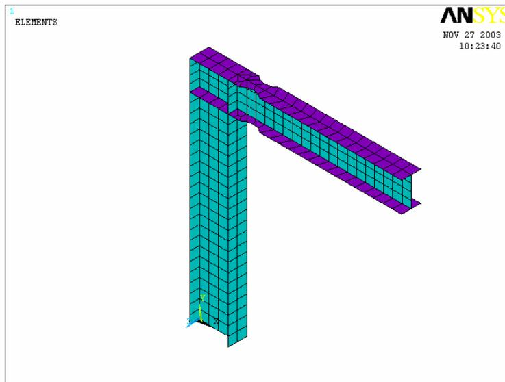
Fig. 6-26 Full Shell Model of Inverted-L Frame with RBS
