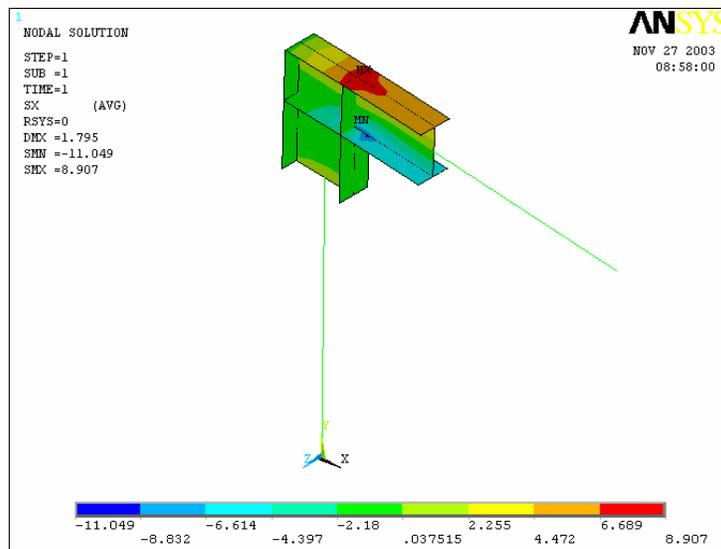
Fig. 6-23 Normal Stress Distribution of Inverted-L Frame
