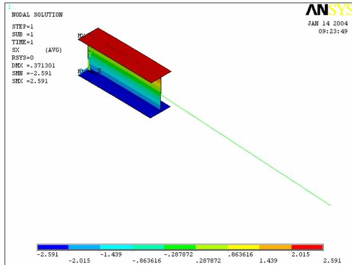
Fig. 6-5 Normal Stress Distribution of Cantilever without RBS under Couple Loading
