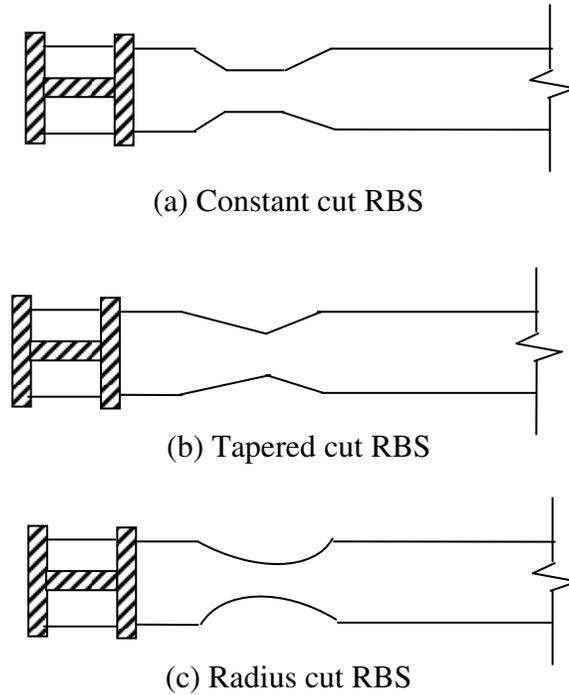
Fig. 2-3 Types of RBS Connections
