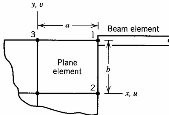
Fig. 3-3 A Plane Beam Element Joined to a Plane Quadrilateral Element [10].
