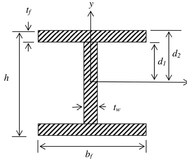
Fig. III-1 Cross-sectional Parameters of an I-Section
