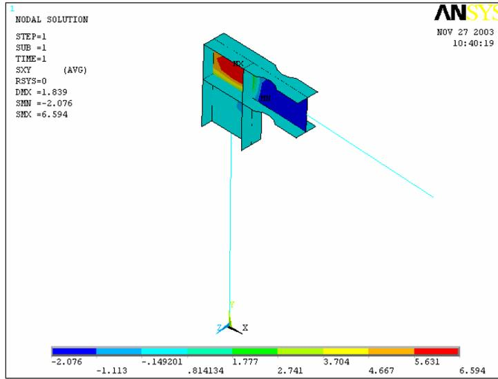
Fig. 6-29 Shear Stress Distribution of Inverted-L Frame with RBS
