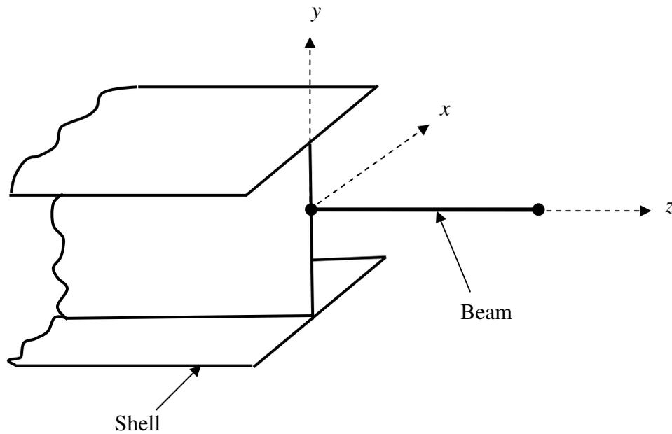
Fig. 5-2 Beam-Shell Model of Wide Flange Beam
