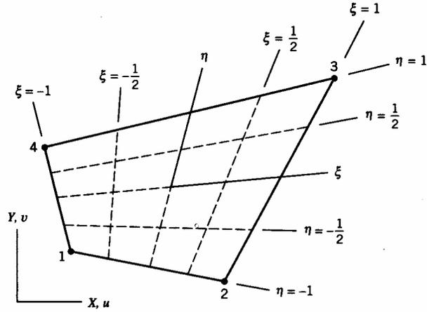
Fig. 3-1 Four Node Plane Isoparametric Element [10]
