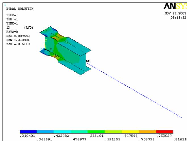
Fig. 6-15 Normal Stress Distribution of Cantilever with RBS under Axial Load
