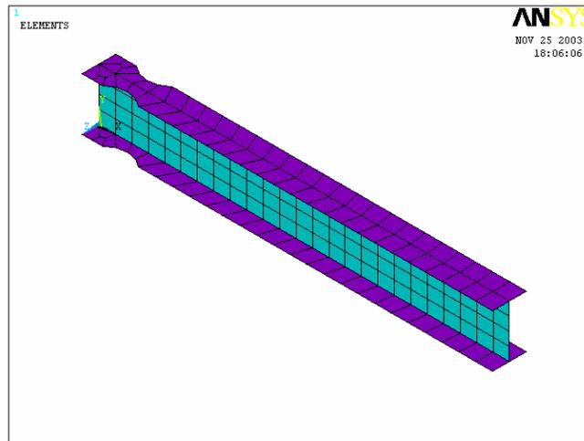
Fig. 6-13 Full Shell Model of Cantilever Beam with RBS
