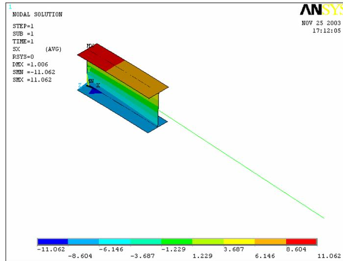
Fig. 6-6 Normal Stress Distribution of Cantilever without RBS under Transverse Load
