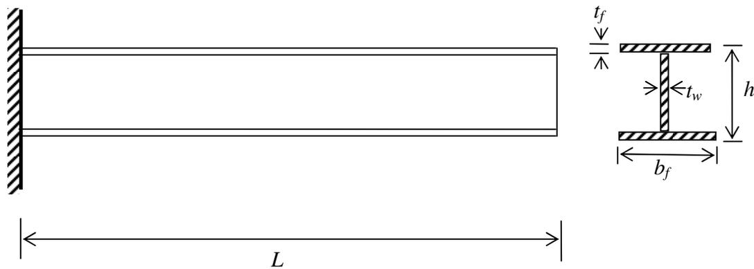
Fig. 6-1 Example 1: Cantilever Beam
