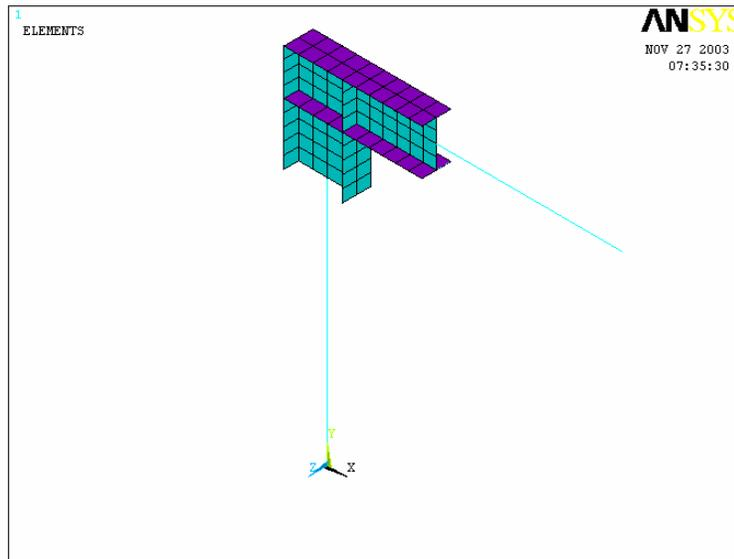
Fig. 6-22 Mixed Model of Inverted-L Frame without RBS
