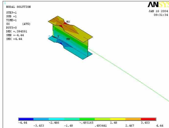
Fig. 6-16 Normal Stress Distribution of Cantilever Beam with RBS under Couple Load
