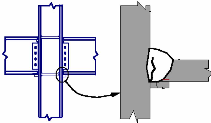
Fig. 2-2 Common Zone of Fracture Initiation [3]
