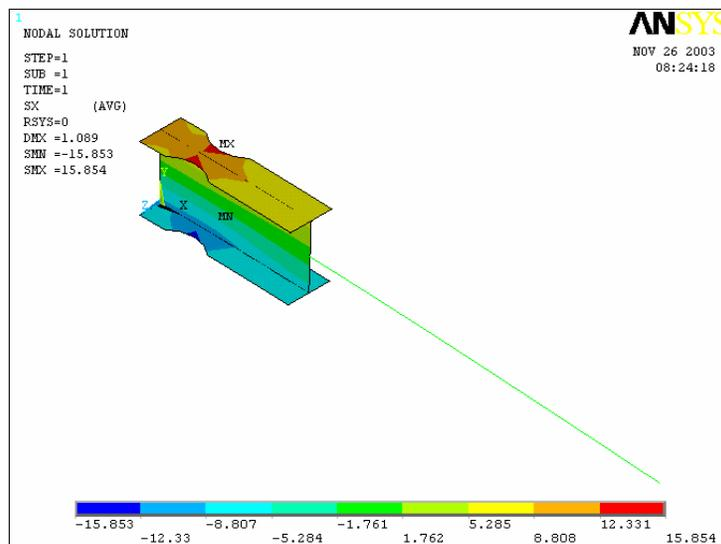
Fig. 6-17 Normal Stress Distribution of Cantilever Beam with RBS under Vertical Load
