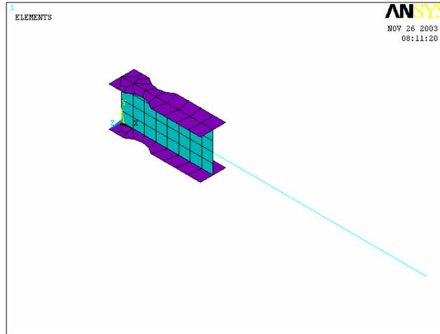
Fig. 6-14 Mixed Model of Cantilever with RBS
