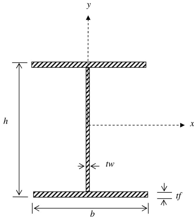
Fig. A-1 Local Coordinate System of I Section
