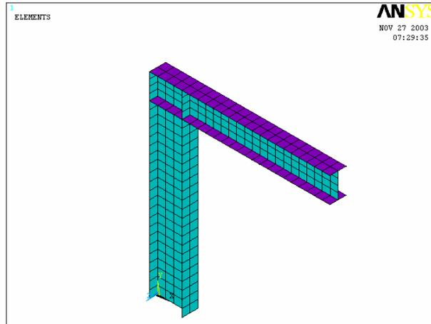
Fig. 6-20 Full Shell Model of Inverted-L Frame without RBS
