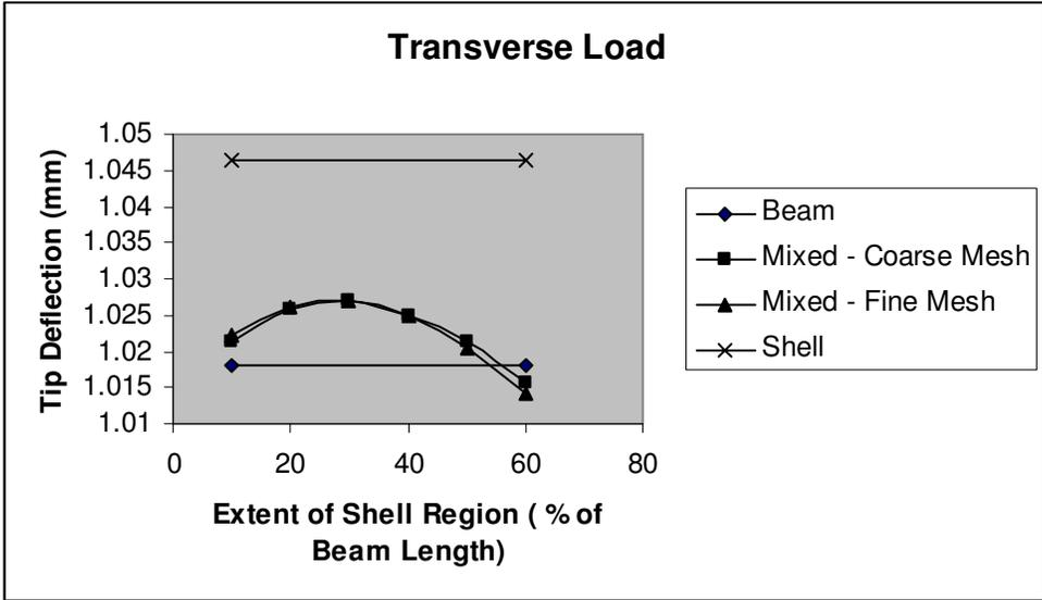
Fig. 6-11 Tip Deflection vs. Extent of Shell Region for Transverse Load
