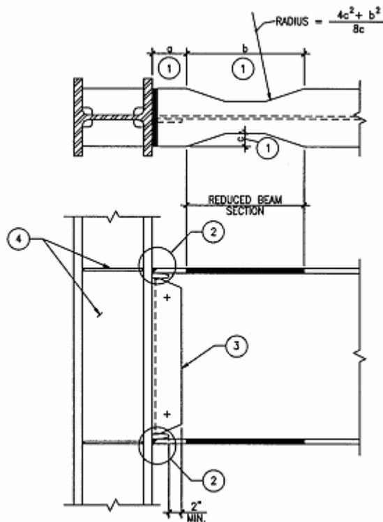
Fig. 2-4 Reduced Beam Section Connection Detail [4]
