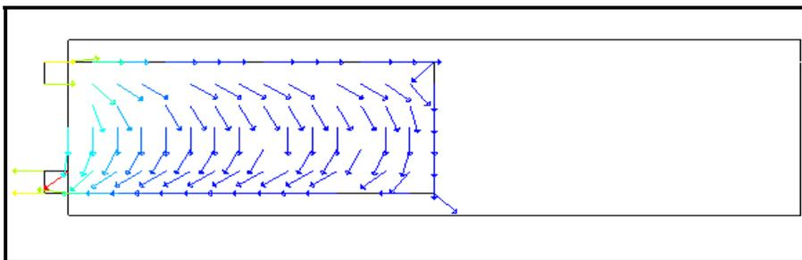
**Figure 4.** Current density distribution in a piezoresistive cantilever subjected to a surface stress.
