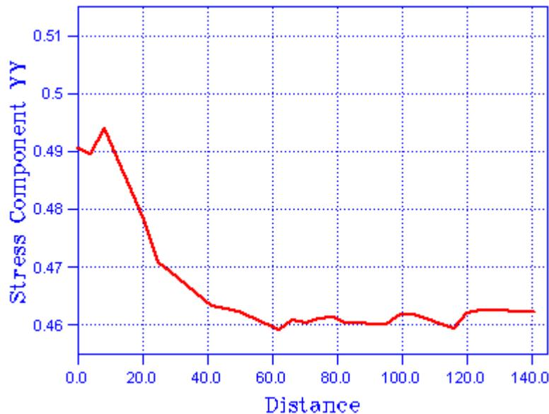
**Figure 11.** Increase in total integrated transverse stress (in MPa) in piezoresistive cantilevers due to structural discontinuities.
