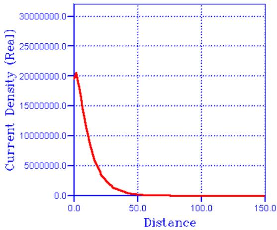
**Figure 5.** Longitudinal distribution of current density ( $\text{pA}/\mu\text{m}^2$ ) in a piezoresistive cantilever subjected to a surface stress.
