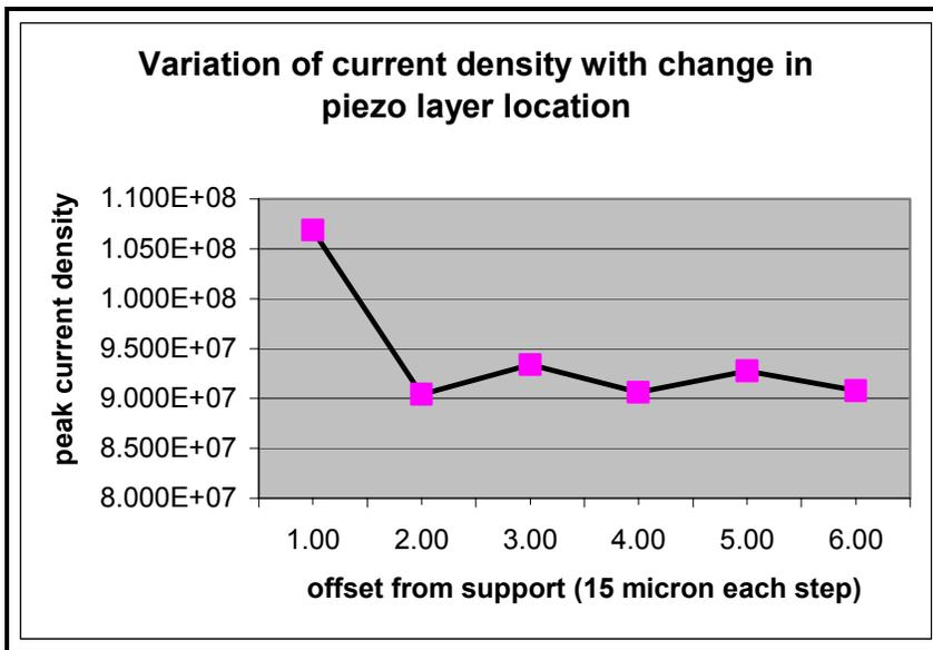
**Figure 6.** Variation of change in current density ( $\text{pA}/\mu\text{m}^2$ ) in a microcantilever with change in location of piezoresistive layer.
