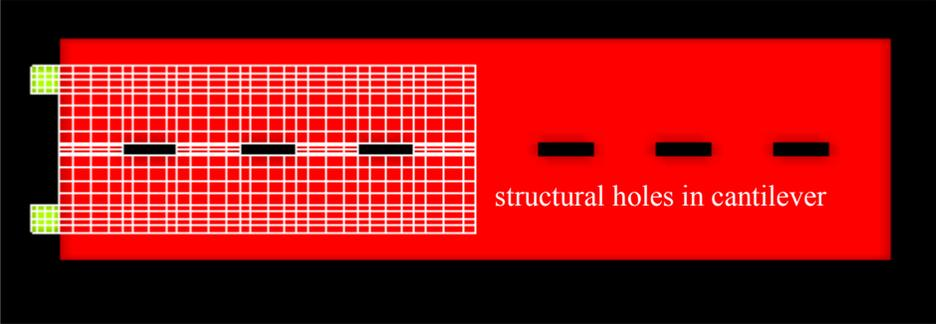
**Figure 8.** Stress Concentration in piezoresistive cantilever device can be achieved through structural discontinuities like holes.
