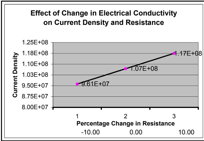
**Figure 7.** Variation of change in resistance in a microcantilever with change in electrical conductivity of piezoresistive layer.
