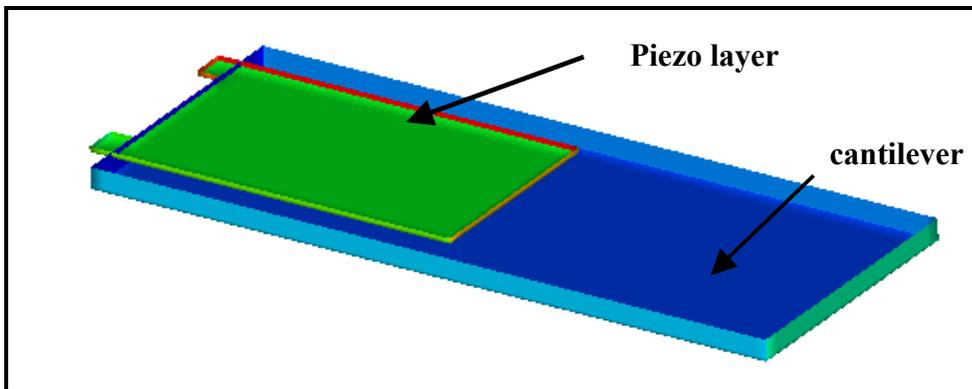
**Figure 1.** Cutaway view of a piezoresistive cantilever device.
